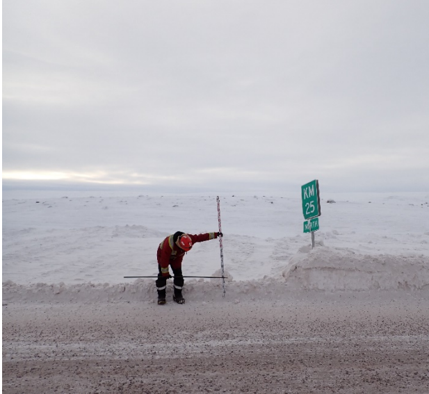
Photo 9-5. Compliant snowbank (40 cm) at KM 25.
