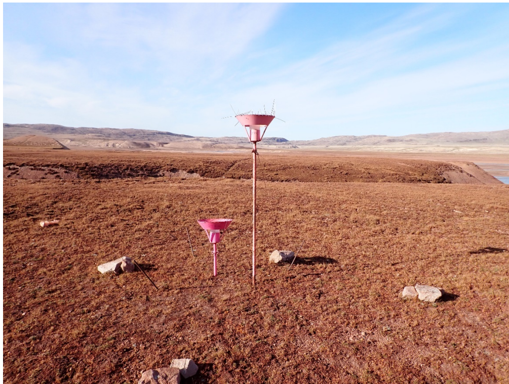
Photo 1. Side-by-side standard (2.0 m) and short (0.5 m) dustfall collectors.
