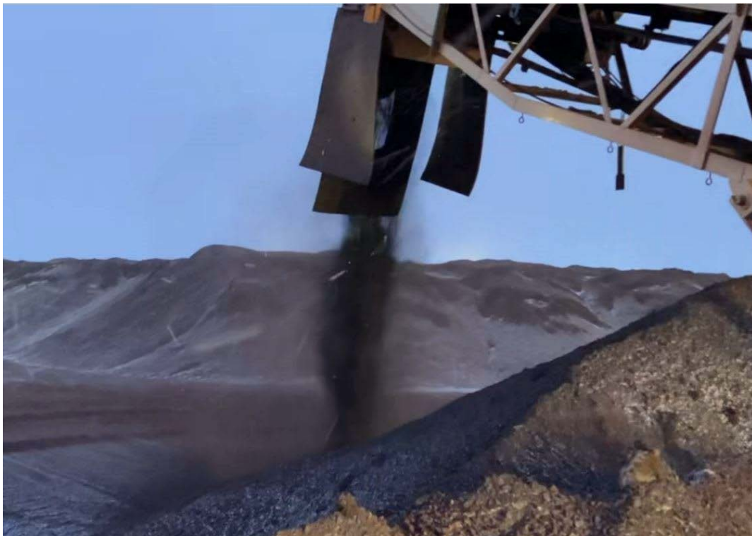
Photo 7-3. Stacker C at the crusher ore stockpile with untreated ore.
