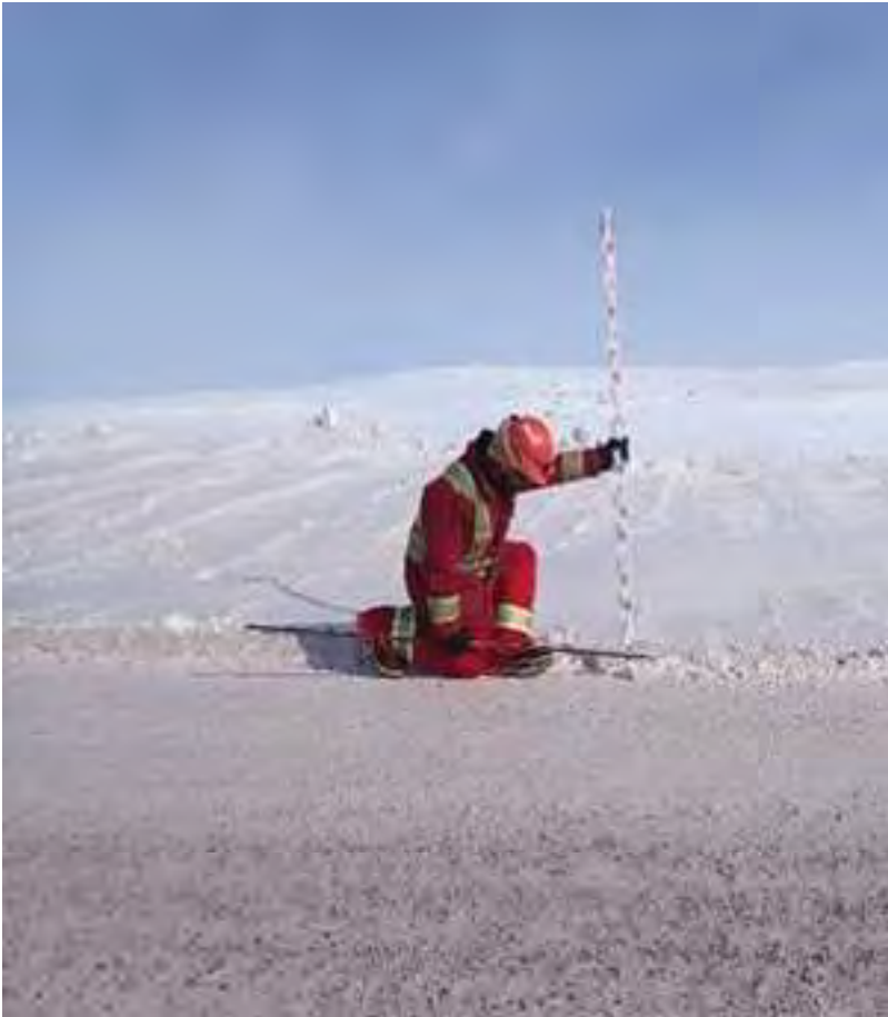
Environmental Field Technician Conducting Snow Bank Height Measurements Along The Tote Road
