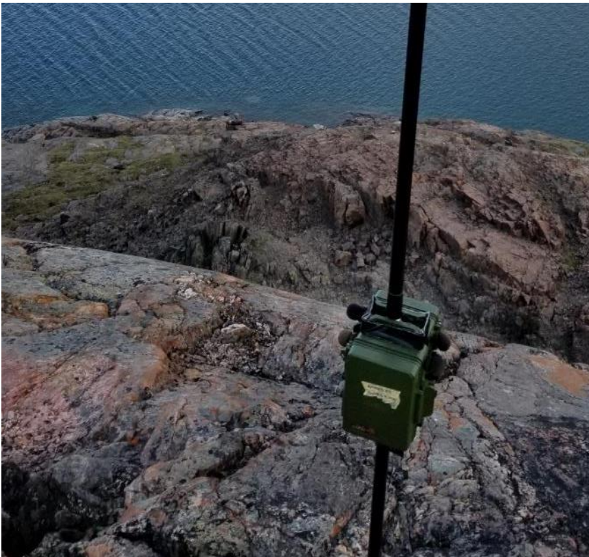
Photograph 4-1: Two SM4 acoustic recorders mounted back-to-back on a fiberglass pole. The shoreline location of the Inuit hunting camp is visible in the background.
