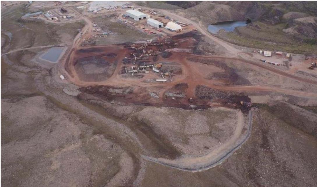
**Photo 25 - Mary River Mine Site Crusher Pad Ore Stockpile and Engineered Drainage Ditch and Sedimentation Pond, July 2016**
